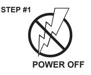
TURN OFF POWER AT CIRCUIT BREAKER to prevent risk of electric shock.
