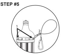
If lamp being installed is over 60w, attach provided tether cable to lamp. Locate either entry hole(1) on lamp shown in diagram and feed looped end of tether cable(2) through hole. You may need to crimp with pliers first. Once through, take end with grappling clip through loop as shown, tighten and secure clip to safe location.
