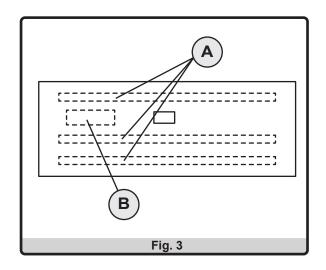
4. Attach the LED magnetic strips (A) to the intended mounting surface, secure each strip with 2 self-tapping screws (AA) at both ends. Check to ensure that no wires or building plumbing are located behind the screw locations. Optional screw anchors (EE) are provided for soft materials if needed.
