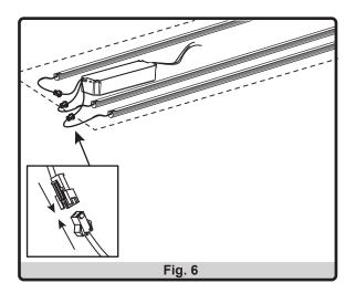
7. Connect the fixture wires to the supply wires -- black to black, white to white, and green to copper/bare.
