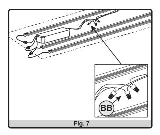
8. Replace any wiring compartment covers or housing pieces so that all wiring connections (wire nuts and quick disconnects) are tucked away from contact.
