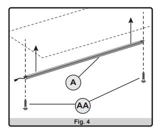
5 . Hold the external driver (B) up against the mounting surface and use a power drill with philips bit to secure the external driver (B) using two self-tapping screws (AA). Check to ensure that no wires or building plumbing are located behind the screw location
